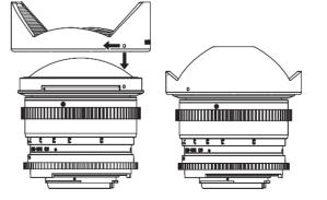
Align the attachment reference point on the hood with the hood reference point on the lens, push the hood onto the lens and turn the hood clockwise until it makes a clicking sound.
